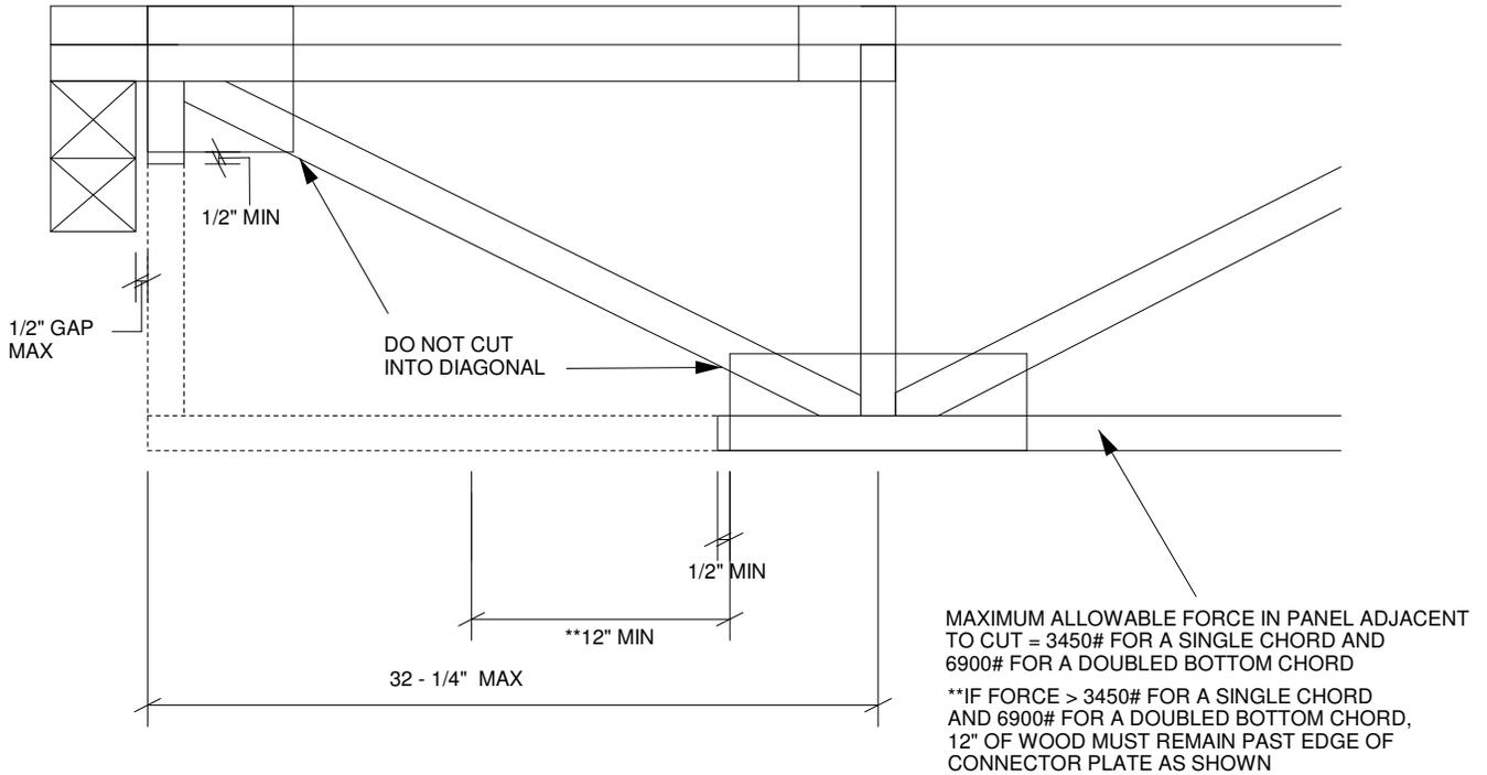
1. LUMBER MUST BE CUT CLEANLY AND ACCURATELY AND THE REMAINING WOOD MUST BE UNDAMAGED.
